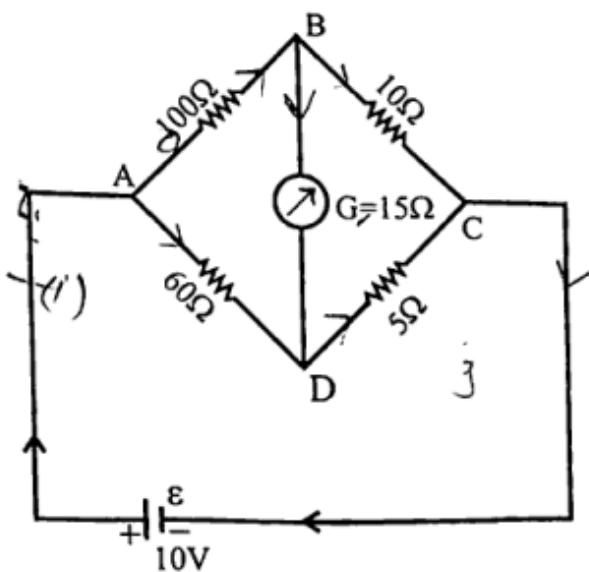
A galvanometer of  $15\Omega$  resistance is connected across BD. Calculate the current through galvanometer when a potential difference of 10 V is maintained across AC.
