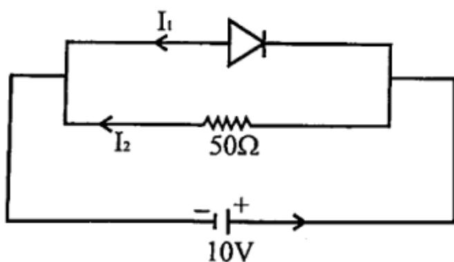
If a diode having infinite reverse-bias resistance is connected in a circuit as shown in the figure, then  $I_1$  and  $I_2$  are respectively
