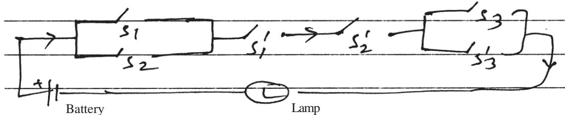
8. Write the following circuit symbolically and construct its switching table. What conclusion would you draw from the table ?
