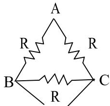
Q. (8) Calculate the resultant resistance between point B and C from the following circuit
