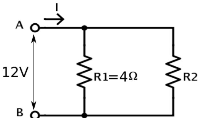
A student has two resistors-  $2\ \Omega$  and  $3\ \Omega$ . She has to put one of them in place of  $R_2$  as shown in the circuit. The current that she needs in the entire circuit is exactly 9A. Show by calculation which of the two resistors she should choose.
